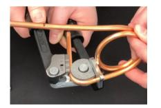
Bend the tube legs using the lever benders
