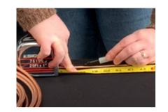
Measure out the copper tube to 24"
