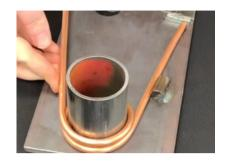
Shape the copper tube using the metal template
