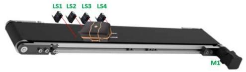
When the 4<sup>th</sup> proximity sensor is activated, if only the 2<sup>nd</sup> and 3<sup>rd</sup> sensor LS2 & LS3) are detecting, this means a Regular luggage is on the sorting belt and the following will occur:
