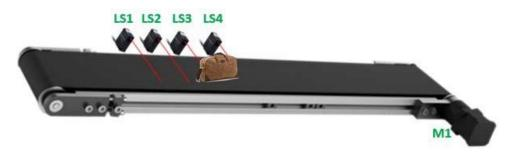
When the 4<sup>th</sup> proximity sensor is activated, if only the 3<sup>rd</sup> sensor (LS3) is detecting, this means a small luggage is on the sorting belt and the following will occur:
