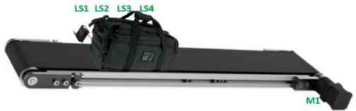
When the 4<sup>th</sup> proximity sensor is activated, if all sensors (LS1, LS2 & LS3) are detecting, this means an over-length luggage is on the sorting belt and the following will occur:
