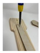
Step Four: Place flipper (#5) on top of base (#1) and screw it into the previously made mark
