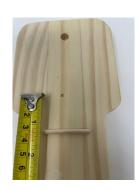
**Step Three:** 1.1/4 inch from mark position round dowel to base.
