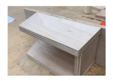
Add the bottom piece using wood glue and nails
