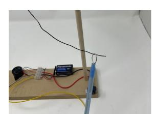
Step 5: **Installing the Wand** Remove the steel wire from the upper hole on the right dowel.
