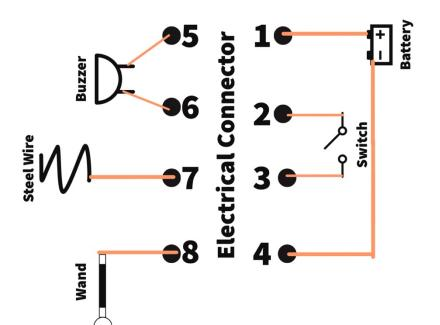
To complete the wiring of the components through the electrical connector taped to the base please follow the steps below and reference the diagram.
