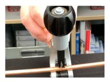
Cut the tube using the tube cutters, being careful not to squash the tube
