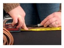
Measure out the copper tube to 24"
