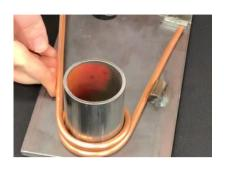
Shape the copper tube using the metal template
