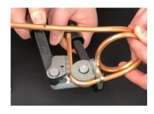
Bend the tube legs using the lever benders
