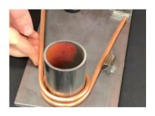
Shape the copper tube using the metal template
