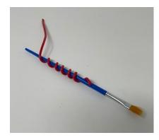
Step 6: **Coiling Wires**Using the paint brush handle wrap the wires around it to create a wire coil.
