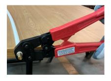
Crimp the ring into place using the crimp tool
