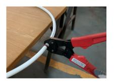
Crimp the second ring into place using the crimp tool
