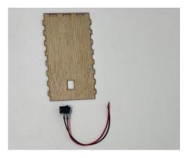
Step 3: Installing Switch Locate the side with the square opening, put the wire through the opening and push the switch in place to secure it
