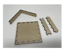
Step 2: The Base Assemble the four sides and insert them into the base and secure them in place with a small amount of glue
