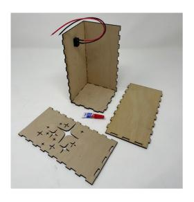
Step 4: **Night Light Assembly** Identify the top piece (small square) the box is built on a tongue and groove system. Insert the four sides into the top piece. Secure with glue
