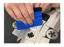
Slowly peel back the decal using the squeegee to remove any air bubbles
