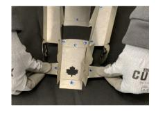
Fold the sheet metal along the seam, in corresponding order
