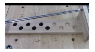
**Please Note:** If your boards did not come pre-drilled, you will drill holes on the rear board for the rod pockets, 1.4in from each side, the front and rear cap holes will be drilled at 0.75in from each sides end. The front and rear boards should be centered to the baseplate and then drilled and secured with screws.
