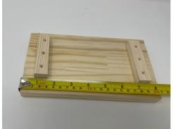
**Step 1:** Take the 3 Tabletop Pieces (A) and place them upside down (rounded side down), measure 1 inch, and secure the brace (B) with screws (G) on each side
