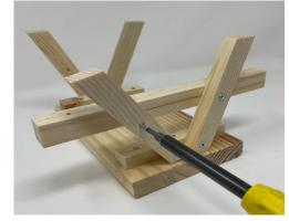
Step 3: Next install the seat supports (D) place the support inside of the legs and screw into the predrilled holes on the legs into the side supports.
