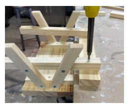
**Step 4:** To install the seats (E) it's best to place the seat upside down (rounded side down) on the edge of your workstation, then with the picnic table upside down, place the seat supports onto the seats and secure in place with screws into the predrilled holes
