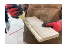
Apply glue to the rabbets and add the front to the bottom piece using nails
