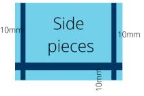
Identify the layout on the side pieces (10 mm in from the bottom and sides of the piece)
