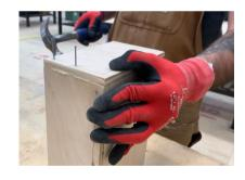
Assemble one side, the back piece and additional side piece
