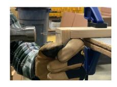
Nail the 2 pieces together using a hammer
