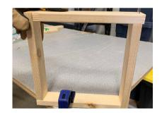
Repeat the process for all 4 sides. Overlap the end of each piece of wood with the end of the next as shown
