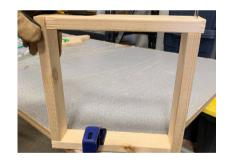
Repeat the process for all 4 sides. Overlap the end of each piece of wood with the end of the next as shown
