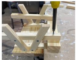
Step 4: To install the seats (E) it's best to place the seat upside down (rounded side down) on the edge of your workstation, then with the picnic table upside down, place the seat supports onto the seats and secure in place with screws into the predrilled holes
