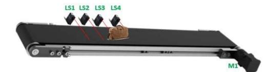
When the 4<sup>th</sup> proximity sensor is activated, if only the 3<sup>rd</sup> sensor (LS3) is detecting, this means a small luggage is on the sorting belt and the following will occur:
