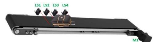
When the 4<sup>th</sup> proximity sensor is activated, if only the 2<sup>nd</sup> and 3<sup>rd</sup> sensor LS2 & LS3) are detecting, this means a Regular luggage is on the sorting belt and the following will occur:
