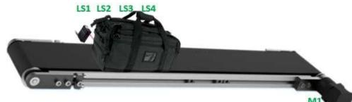
When the 4<sup>th</sup> proximity sensor is activated, if all sensors (LS1, LS2 & LS3) are detecting, this means an over-length luggage is on the sorting belt and the following will occur:
