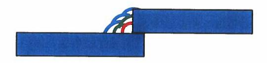
FINISHED WELD SHOULD BE SLIGHTLY CONVEX WITH AS MANY PASSES AS NEEDED TO ACHIEVE DESIRED APPEARANCE.
