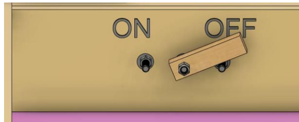
Figure: ECU Breaker Switch
